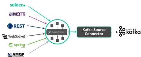
The source connector uses Solace's high performance Java API to move PubSub+ data events to the Kafka Broker. PubSub+ supports popular messaging APIs and protocols like AMQP, JMS, MQTT, REST, WebSocket and more so the connector can move any message to a topic (keyed or not keyed) on the Kafka broker.
